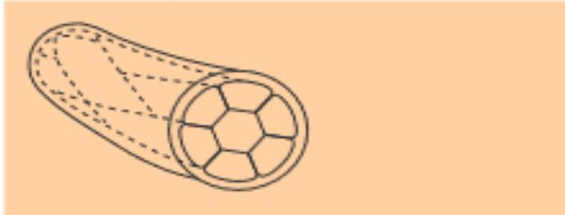
*The thread interior (the so-called thread core), a bundle of parallel filaments, is imbedded in a mantle-like or tube-like coating that provides a smooth cover.*
